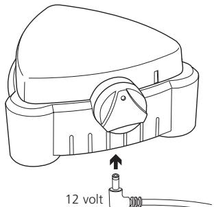
5. Rotate the control knob **clockwise** to adjust the stirrer speed between 350-2000rpm.
